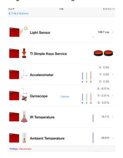
Turn on and off the sensors by selecting '**Profiles**' in the bottom, left corner on iOS or click on '**Services**' on Android. In the Profiles section on iOS it is possible to adjust the sensor data collection interval by moving the sliding bars, and select which axis to display for the multi-axis sensors. When you click '**Back**' the TI *Bluetooth* SensorTag app will display the selected sensor data with the selected data interval.
