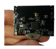
Note that when inserting the battery for the first time, the PCB contact point surface may have a thin layer of solder residue that can prevent contact with the battery. Remove and insert the battery a few times to power the SensorTag.
