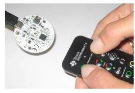
Touch link the Zlight2 boards by holding the remote control close and simultaneously pressing the "on" and "off" buttons
