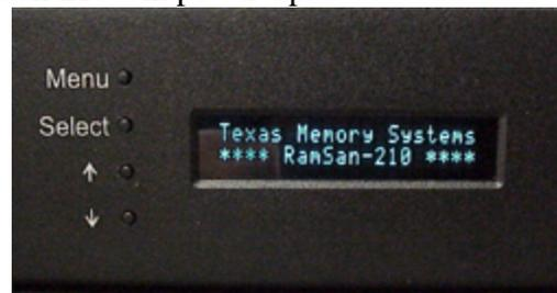
3. After the firmware has finished booting, the front panel display will indicate “Bringing Disks Online”. The system disks take approximately 10 seconds each to spin-up.
