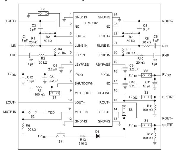
Figure 3-3. TPA0202 EVM Schematic Diagram
