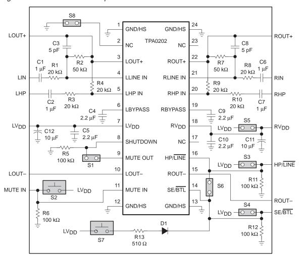
Figure 3-5. TPA0202 EVM Jumpers and Switches
