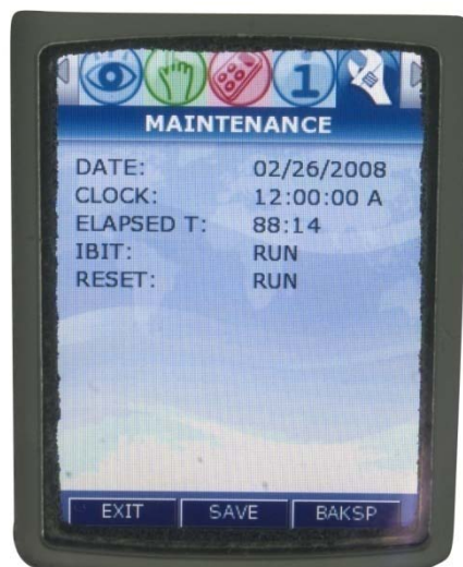
Figure 4-1 Maintenance Menu Screen
