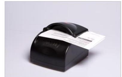
3. During reading, the document must lie flat against the document window. The leading edge of the booklet or card should be all the way to the back of the document window (and underneath the document clip, if installed). The left edge of the booklet must be against the document guide.
