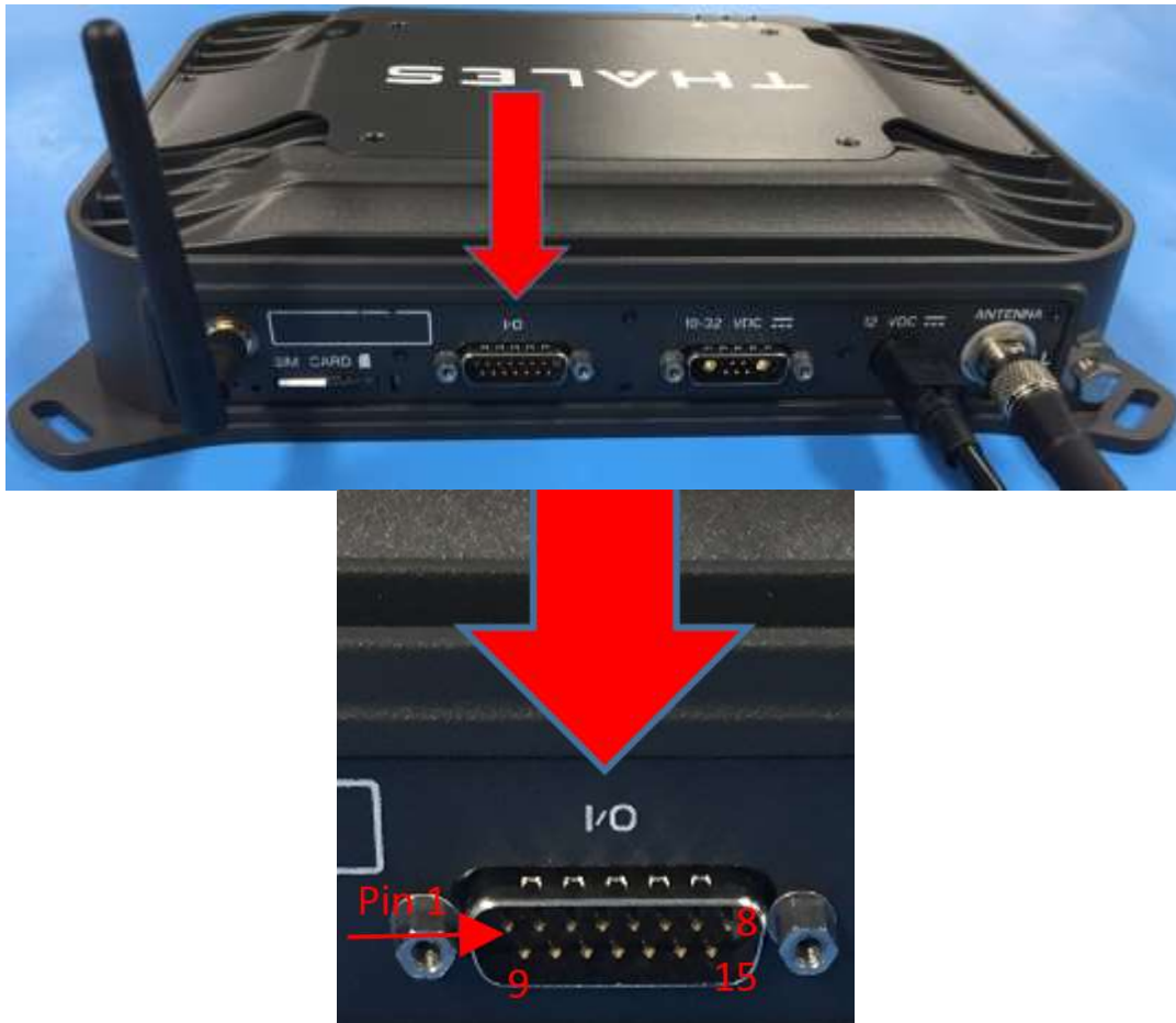
Figure 7-2 GPIO Connector Pin Detail
