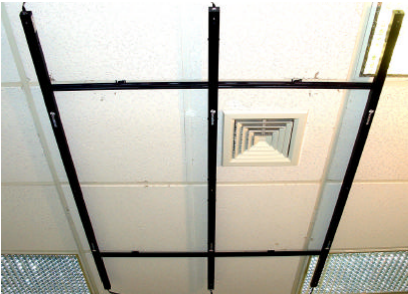
Figure 6 - IS-900 SoniFrame with three 6 ft. SoniStrips Assembled and Mounted on a Ceiling
