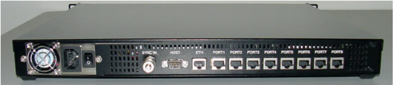
Figure 44 - Back Panel of IS-900, SYNC IN is External GENLOCK Input
