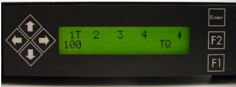
Figure 39 - Tracking Quality Status for a Wired Tracking Station 1
