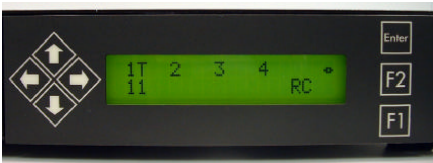
Figure 35 - LCD Panel in Normal Display Mode (Tracking One Station)
