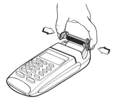
Place the roll of paper in the casing, paper output towards the pin pad. Leave a few inches of paper outside.
