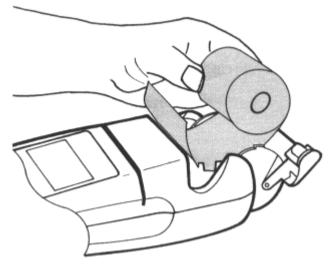
Close the printer casing. You will hear a "click" sound to confirm the casing is closed.
