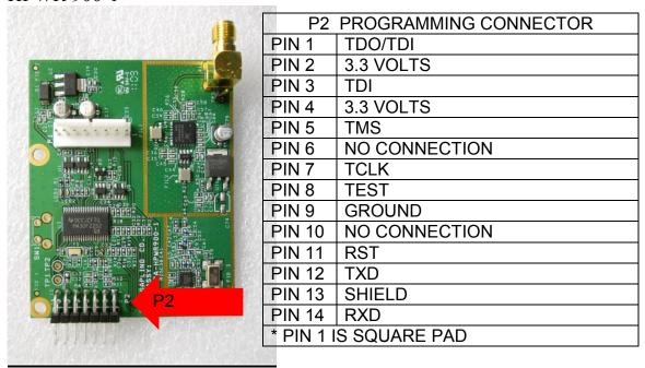
HPWR-900-1 RF module as a remote antenna, to be connected to a Sapling Master Clock.
