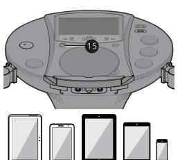
15 Press the ON/STANDBY button to turn the unit off; the On/Standby indicator will light red and the LCD Screen will turn off.
