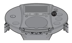
1 1 Press the Auto Voice Control (AVC) button to turn this option On (AVC ON will appear in the screen) and the vocals on a multiplex recording are muted as soon as the singer begins singing into the microphone. When the singer stops singing, the vocals are automatically unmuted.
