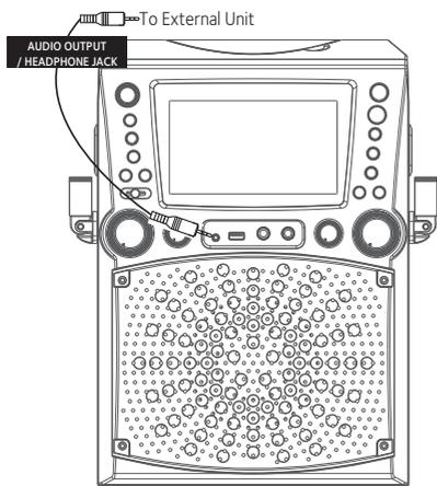
Connect an external device by using an appropriate cable (3.5mm audio cable not included) as shown.
