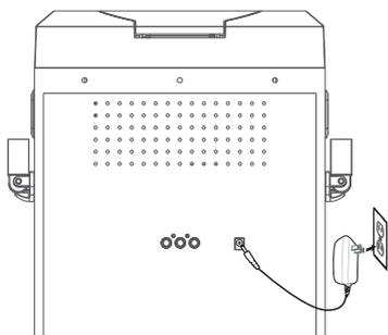
Insert the small end of the AC adapter into the DC IN jack on the rear of the unit. Insert the other end (with the 2 blades) into a conveniently located AC outlet having 120V AC, 60Hz.
