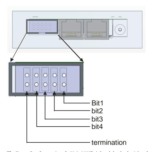
The Contact Interface consists of a 10pin 0.100" pitch male header that is keyed.
