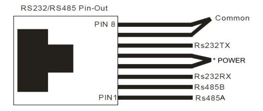
The RJ-45 connector is shown tab side down
