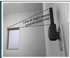
Locate Qrelay pointing up, as far from the floor as possible, within shades' line of sight for best results. The best position may require trial and error.
