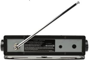
You can use a variety of antennas. To connect an external antenna, follow the installation instructions supplied with the antenna. Always use 50-ohm coaxial cable, such as RG-58 or RG-8 low-loss dielectric coaxial cable. You may also need a BNC adapter.
