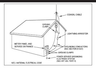
WARNING: Use extreme caution when installing or removing an outdoor antenna. If the antenna starts to fall, let it go! It could contact overhead power lines. If the antenna touches a power line, touching the antenna, mast, cable, or guy wires can cause electrocution and death. Call the power company to remove the antenna. DO NOT attempt to do so yourself.
