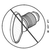
Use of this POL transport plug (plastic part with external threads)
