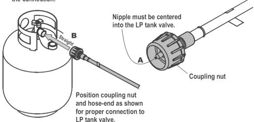
6. Turn the coupling nut clockwise to tighten to a full solid stop. The hose-end will seal on the back-check feature in the LP tank valve, resulting in some resistance. An additional one-half to three quarters turn is required to complete connection. Tighten by hand only - do not use tools.
