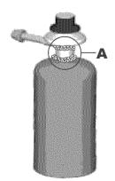
▲ If growing bubbles appear, there is a leak. Retighten connection and repeat steps 1 and 2
