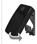
Secure the reader module to the backplate using the M3x10mm screw supplied.
