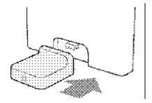
Slide open the battery compartment on the back of your TH25/TC28330PE1 Handset. Insert the 2 x AAA rechargeable batteries supplied. Slide back the cover to close.
