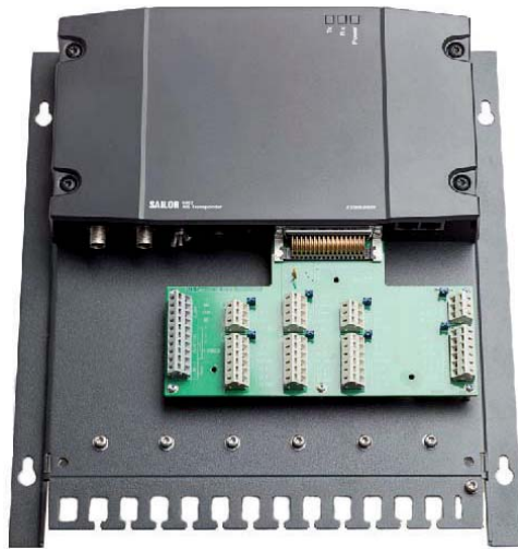
Figure 2-6: SAILOR 6283 AIS Connection Box and Wall Tray
