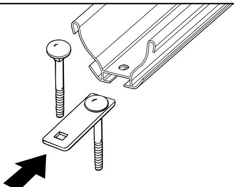
**b. Drops carriage bolts into washer plate.**
