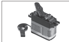
8128 Digital Speed Servo 12.5Kg-cm@6V,DS1313
