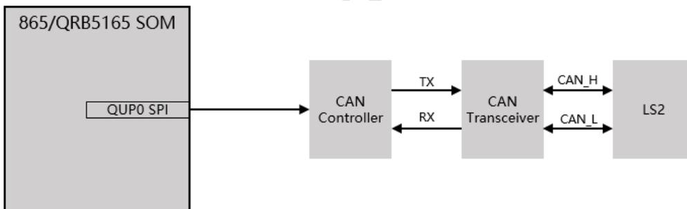
The CAN signals are rounded from CAN transceiver which is from SPI translation. The signals are:
