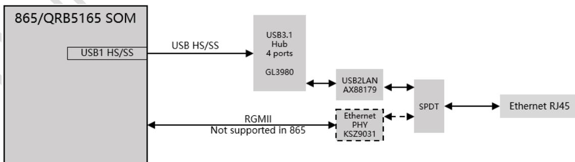
RB5 has the translation from USB1, a USB HUB and a USB to Gigabit Ethernet controller. RB5 uses an RJ45 (see Section 1.2.1, #9) as the physical interface.
