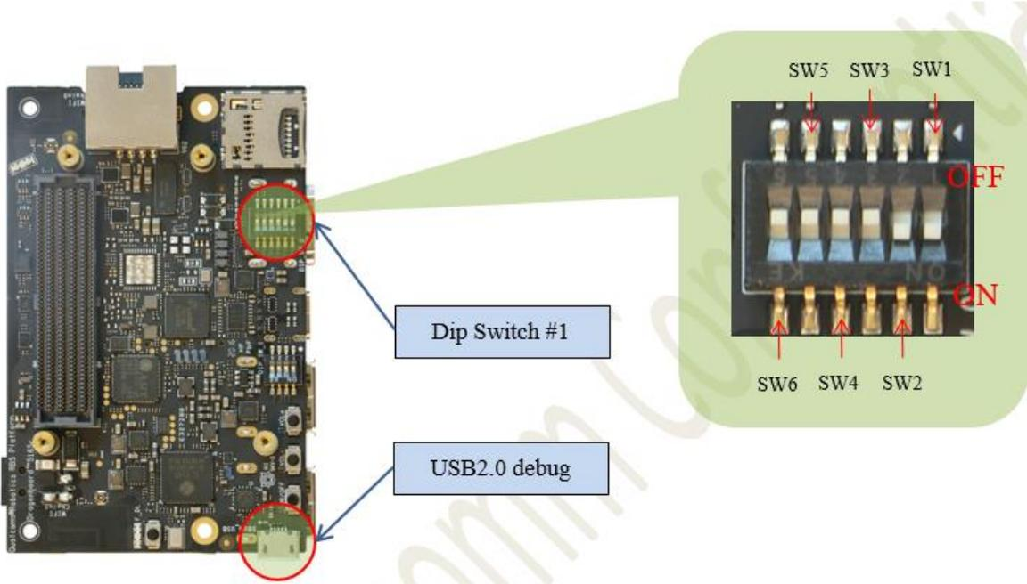
4. Connect the USB cable Micro-B plug to the USB2.0 debug port (see section 1.2.2, #21), and connect the other end to an available USB port on the host PC.
