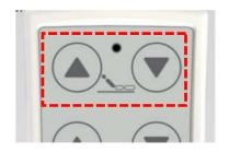
C. TH30: Keep pressing button 1 and button 2 for 5 seconds to activate pairing mode. Wait until the LED indicator keeps flashing slowly.
