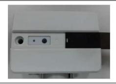
D. TRF2: Keep pressing reset button till LED indicator flashing 2 times. This indicates the pairing procedure completed. (the LED indicator on TH30 would flashing 2 times at the same time as TRF2s')
