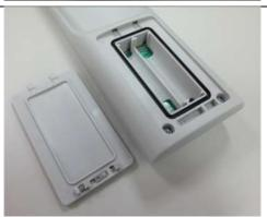
II. Put battery cover and lock it after replaced 2×AA batteries.
