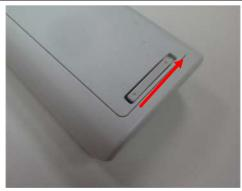
Follow the direction of red arrow slide the latch to unlock battery cover.
