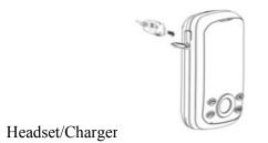
During charging, the battery capacity icon on the screen flickers from the right to the left. After the battery is charged full, the icon is full of bars. Slight heat during charging is normal.
