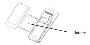
Note: Do install the battery as per the diagram so as prevent the battery contact patch being damaged.
