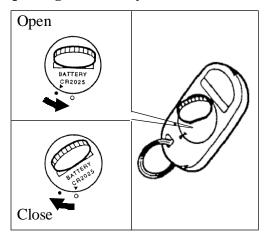
When the Remote Keyless Entry Transmitter's Battery begins to get weak, it may take several pushes on the button to lock or unlock the doors, and the LED will get dim.
