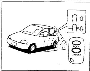
Push the "LOCK" button or, the transmitter to lock the all doors. Be sure the doors are locked after you operate the "LOCK" button. Push the "UNLOCK" button on the transmitter one (1) time to unlock the driver's seat door. Push the "UNLOCK" button on the transmitter again to unlock the all doors within about 5 seconds after the "UNLOCK" button is first pushed. The doors will automatically lock again if no door is opened within about 30 seconds after the "UNLOCK" button is finally pushed.
