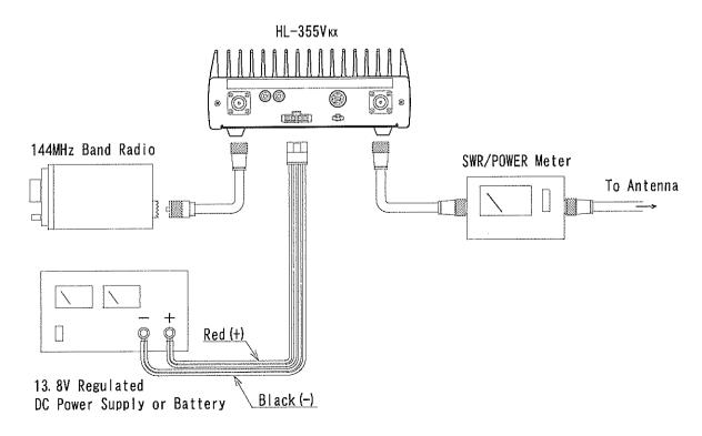
This figure shows the basic connection when RF-key is chosen. When hard-key is preferred, control cable from the proper accessory pin of the radios should be plugged to either ACC1 or ACC2.
