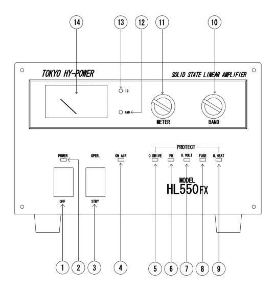
**①POWER** : Main power switch to turn AC power on and off.
