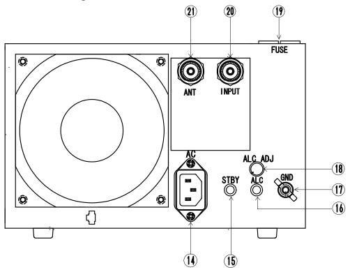
**@AC POWER** : AC Mains Socket. Socket for the AC power cord. (Socket is EMI
