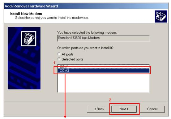
Select the COM port that you have installed "CP210x\_VCP\_Win2K\_XP\_S2K3" driver. For example: COM3 in the installation demo.
