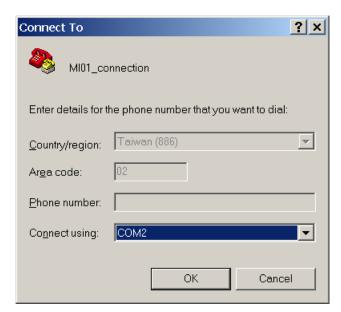
Select the appropriate setting for MI01 data modem serial port setting; then select APPLY/OK.
