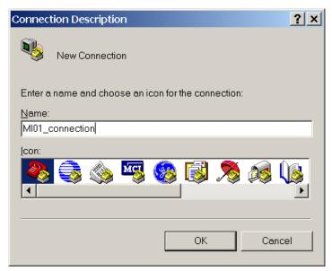
Set the name for connection (e.g. "MI01\_connection"), then press OK Select the PC serial port (for example COM2), then press OK
