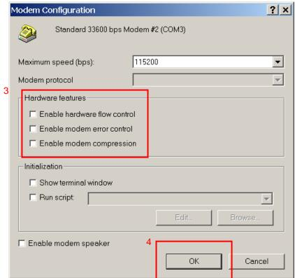
All hardware features of modem protocol should be disabled. Now, you have completed all modem and network setting. You can use Section 2.3 to dial up network directly in the future.
