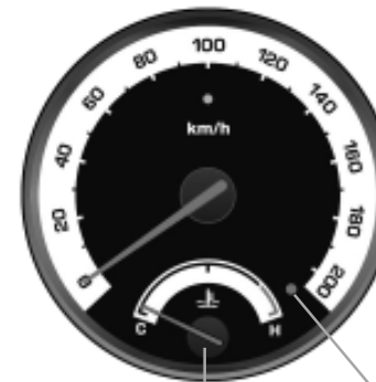
Temperature Gauge High Temperature Warning
