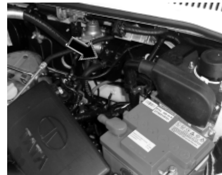
Fuel Filter on LPG System
