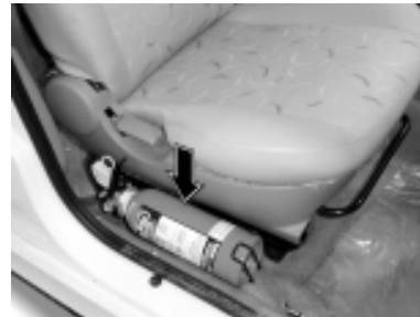
Fire extinguisher near Driver's Seat
