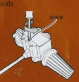
2-Install 1 fresh 9-volt battery as shown. Replace battery cover and re-tighten screw.
