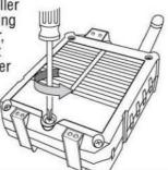
2.Install 2 fresh AAA batteries as shown. Replace battery cover and re-tighten screw.
