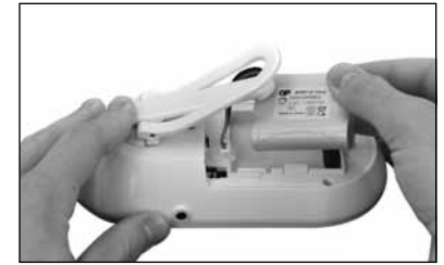
hold belt clip open to install battery pack
