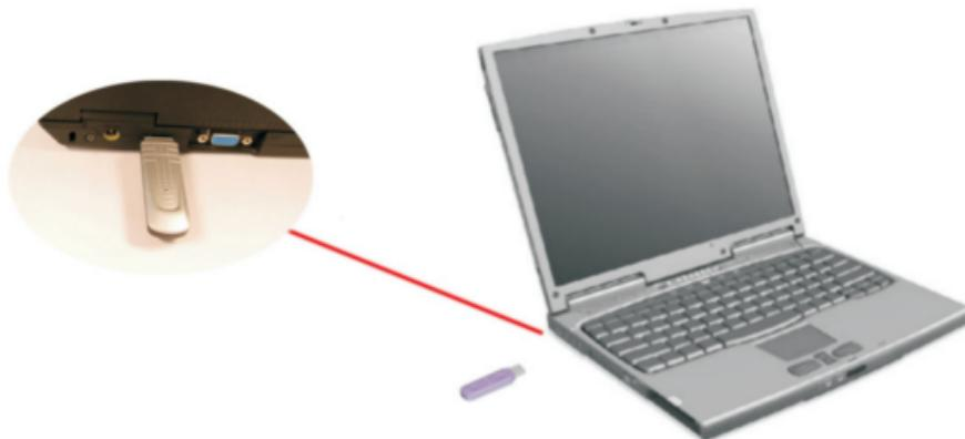
Windows recognises the receiver by the Plug&Play function and initiates the driver installation.
