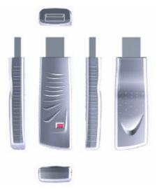
Note that the Channel button (Red button) on the receiver should flash any time the Cordless device is moved or a button is pressed. Then, it will remember your product ID and Channel ID
