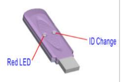
1-2 When the remote near the receiver, press the M-key and Composite Switch together at least 5 seconds (The M-key green LED and Receiver's red LED will be flash then already change a new ID).
