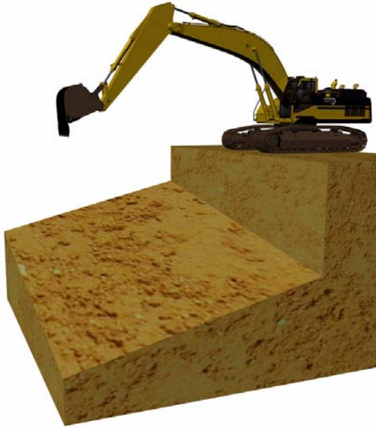
Figure 2-8. Dual Slope Surface
