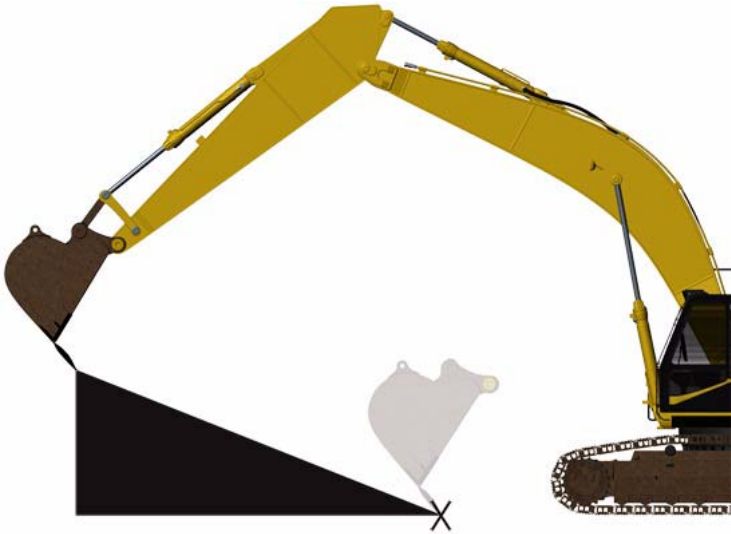
Figure 2-13. Bucket-defined Single Slope Surface
