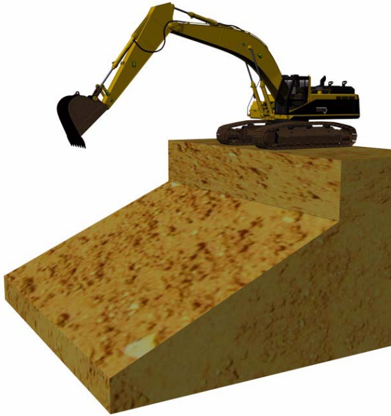
Figure 2-7. Single Slope Surface
