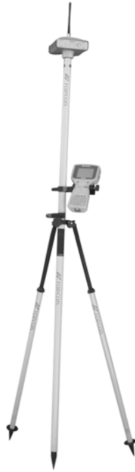
Figure 3-11. HiPer+ Rover Station Setup
