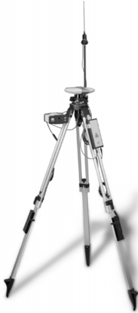
Figure 3-6. Legacy-E Base Station Setup
