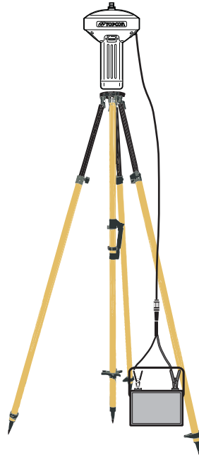
Figure 16: Connect an Auxiliary Battery and the Receiver
