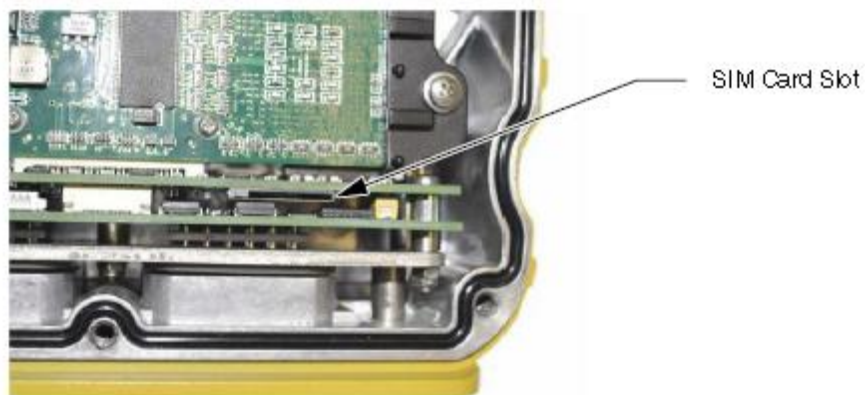
Figure 4. Insert SIM Card
