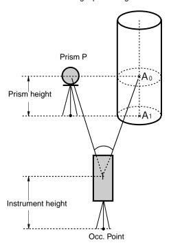
When measuring coordinates of ground point A<sub>1</sub>:Set the instrument height/prism height.
