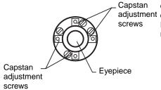
3)Shift the vertical cross-hair line and coincide it with Point D, by revolving the left and right capstan adjustment screws with the adjusting pin.Upon completing the adjustment, repeat the checking adjustment operation once more.
