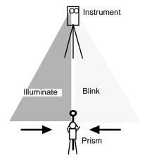
Once you have determined that both of the LED's are equally bright, you are on-line with the instrument.
