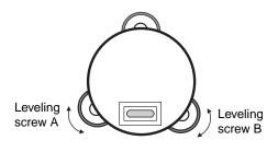
2 Rotate the instrument 90° (100gon) around its vertical axis and turn the remaining leveling screw or C to center the bubble once more.
