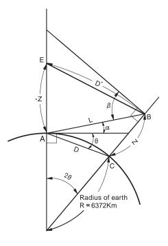
The conversion formula for horizontal and vertical distances is as follows when correction for refraction and earth curvature is not applied.
