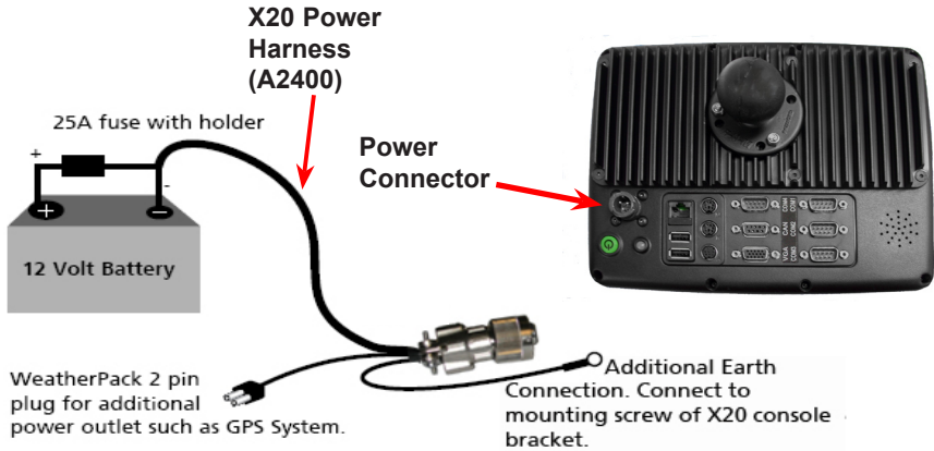
Figure 4-2. Layout of the X20 Power Harness
