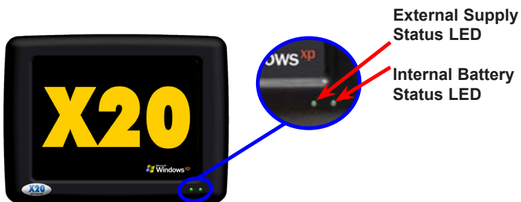
Figure 5-1. LED's Indicating Power Status
