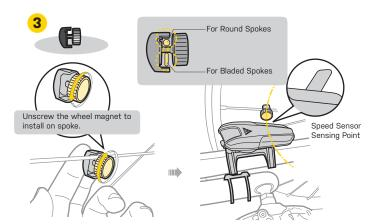
Tighten the Wheel Magnet onto spoke and align with sensing point on sensor.
