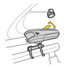
Adjust angle and position of sensor to achieve recommended magnet distances and aligning sensing points.
