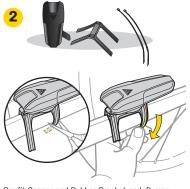
Pre-fit Sensor and Rubber Bracket on left rear chainstay (non-drive side) and trim excess rubber from bracket. Insure the Topeak logo is facing up Install zip ties loosely to allow sensor placement.
