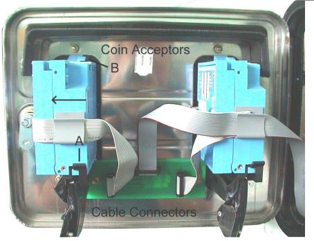
Microcoin electronic coin acceptors are fitted to the unit. These can be reprogrammed by the operator using a hand held programmer. This is available from Tornado either to purchase or on loan. Please contact the Service Department for details. There are no user serviceable parts in the coin acceptors. They should be returned to Tornado for service.
