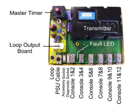
The transmitter motherboard is housed in the master console behind a glass fibre cover. It is accessed by opening the door under the driving controls and removing the glass fibre cover, through the coin acceptor door. Mounted on the transmitter motherboard are the following components
