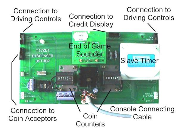
The console motherboard is mounted in the centre of the console and is accessed by opening the coin acceptor door. It is the distribution centre for the console and has the following parts mounted on it.
