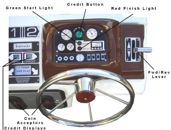
The driving controls are mounted on top of the console and comprise of a control for each function of the model. Each boat uses two channels of the transmitter for its operation. One for the left hand motor and one for the right. Because we use the direction of rotation of the motors to control the direction
