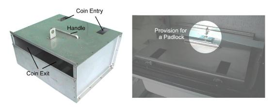
The cash box is mounted in the centre of the console behind the coin acceptor door. There is provision to fit your own pad lock for added security. The cash box is removed from the console by opening the coin acceptor door, removing the padlock if fitted and lifting out using the handle.
