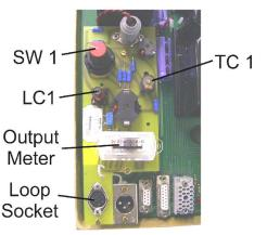
Rotate SW1 fully anti-clockwise and observing the loop output meter select each clockwise position in turn, noting the loop output meter reading at each position. Note: If the loop output meter should read over 10 during this procedure adjust LC1 to return the needle to 5. Please read the note and instructions below before doing this.
