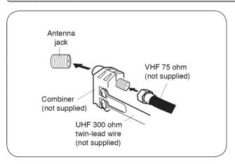
Connect the VHF 75 ohm cable and UHF 300 ohm twin-lead wire to the combiner (not supplied). Attach the combiner to the antenna jack on the back of the TV/DVD.
