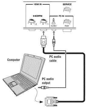
The HDMI 1 input can accept and display VGA, SVGA, XGA, 480i (60Hz), 480p (60Hz), 720p (60Hz), and 1080i (60Hz) signal formats. For detailed signal specifications, see page 49.
