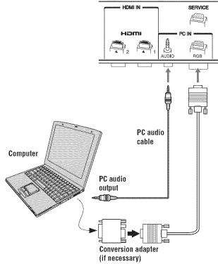
To use a PC, set the monitor output resolution on the PC before connecting it to the TV. The following signals can be displayed:
