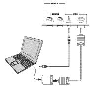
**Note:** Because the PC Audio input is shared with HDMI 1. If **INPUT** source is set to "**HDMI 1**," And the **HDMI 1** signal is DVI format. This PC Audio input will apply for HDMI 1. (Also see item 2 on page 11.)
